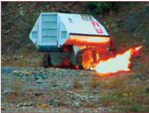
PMA 1 fired under Digger chain
