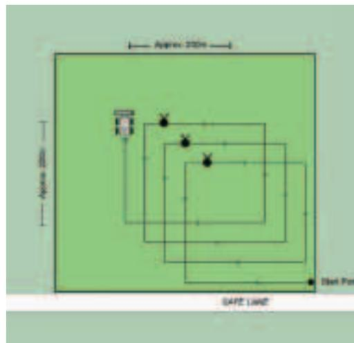
Rolling area using concentric box pattern where mines were not expected but were subsequently encountered. In this example, an approximate mine pattern is revealed. Rolling should stop and clearance assets take over.
