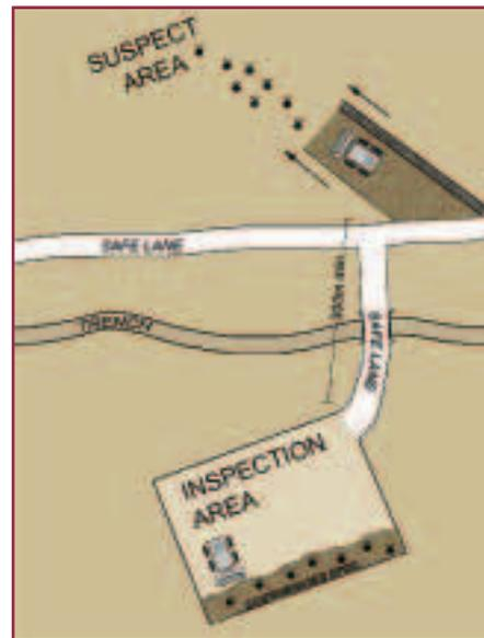
3. Suspect soil is processed to separate mines/UXO from soil. Once this is achieved, ordnance is destroyed by explosive ordnance disposal (EOD) staff. The method of soil excavation and processing depends upon the machine used:
