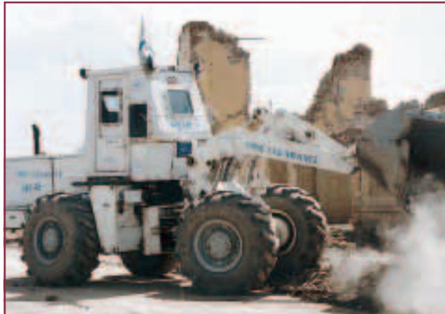
Fig. 17. Converted (armoured) Russian RABA front-end loader conducting rubble clearance, The HALO Trust, Kabul, 1998.
