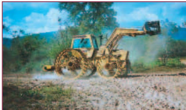
Fig. 30. Pearson Engineering SDTT. The Pearson Roller is attached to the tractor. Used in Thailand.
