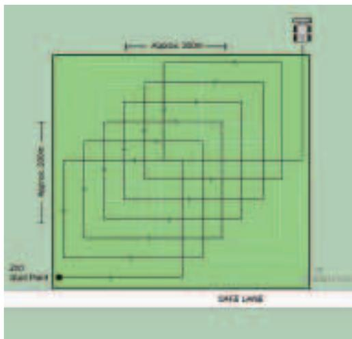
Phase 2 of HALO Trust rolling operation. Grey lines are pattern from first roll. Concentric box pattern ensures that the middle of the area is rolled four times from four directions.
