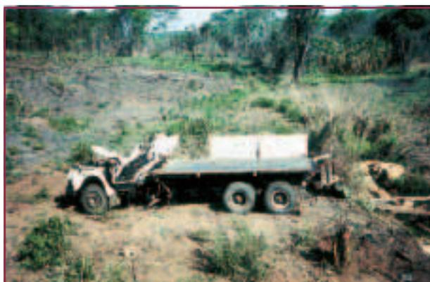
The cab was destroyed with little or no damage towards the rear of the vehicle or the lower left hand side in front. The driver of the truck was killed instantly.
