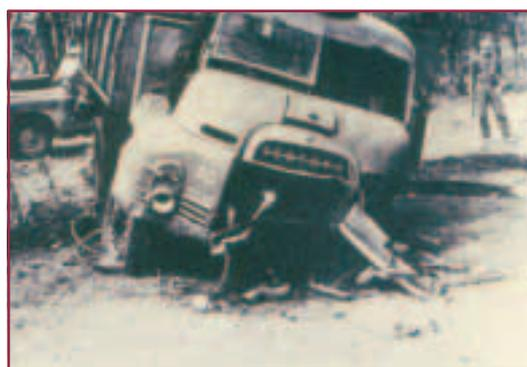
It was previously thought that the water absorbed energy by being converted into spray and vapour, but recent studies suggest that the water, being much heavier than the air in the tyre, deflects the shock wave sideways thereby flattening the cone of destruction.
