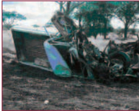
The effect on the occupants depends on their position relative to the detonation point. If an occupant is positioned within the cone of destruction, death is almost certain.
