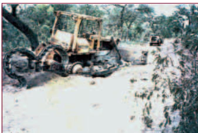
*After some of the roads were cleared by manual teams in Mozambique this was the fate of road-building equipment following them up. Hand-held metal detectors and prodding sticks were cleaning to a depth of some 100mm. The TMA-2 mine detonated after the blade had removed enough cover. The mine was too deep for other vehicle traffic to detonate it.*
