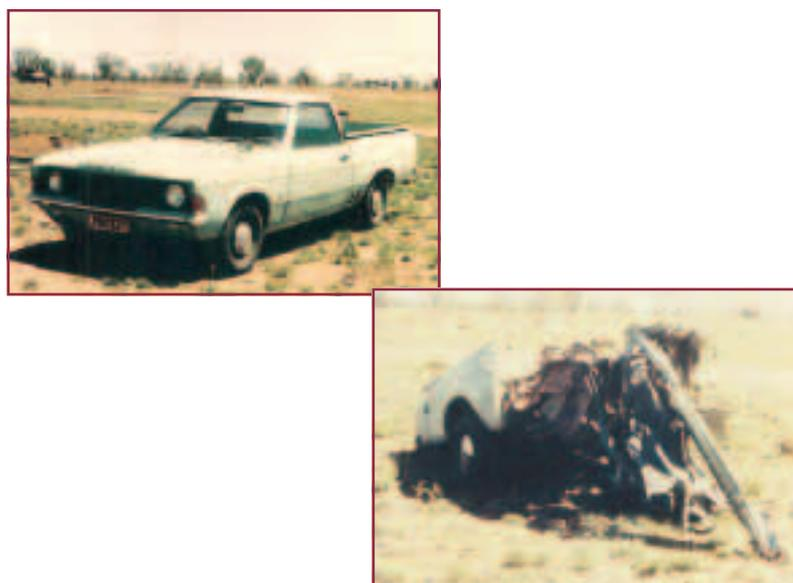
When multiple mines are stacked (either double or triple), the ensuing blast effect on the vehicle, even for a detonation under a wheel, is much bigger due to the increase of explosive charge. Figure 13 depicts a light unprotected vehicle almost completely destroyed by a double mine. The mine detonated underneath the right front wheel. All five occupants were killed instantly.
