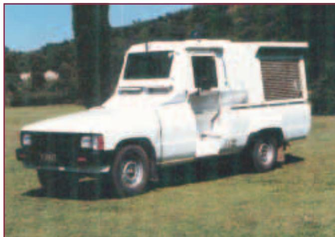
It is also important to prevent the “entrapment” of the blast wave. Lightweight, “blow away” panels should be used in areas within the cone of destruction, such as in the wheel wells.
